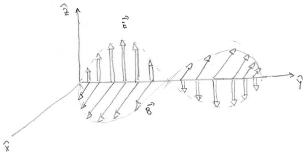
The  $\vec{E}$ , the  $\vec{B}$  and the direction of propagation  $\vec{\gamma}$
