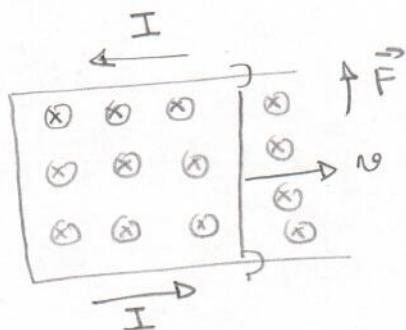
I move a conductor in the presence of a magnetic field. A Lorentz force will set up a current. So moving a conductor in a magnetic field I can convert mechanical energy to electrical energy.
