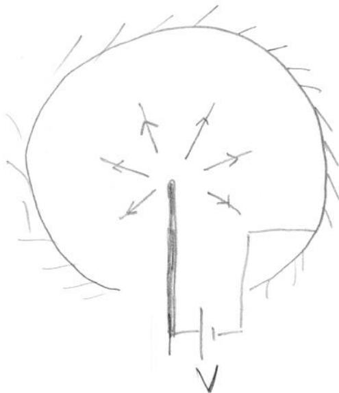
If a small amount of He is introduced in the chamber the He atoms can, by random motion, hit the tip and get ionized. Then the He ion will be moved by the strong electric field, and hit the surface of the bulb. This way the atomic level structure of the tip can be mapped out.
