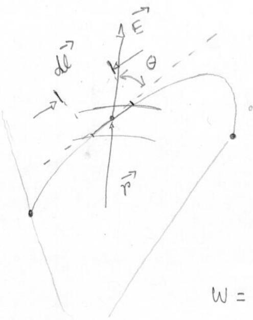
$$\begin{aligned} dW &= \vec{E} \cdot d\vec{l} \\ &= \frac{qV}{4\pi\epsilon_0} \frac{1}{r^2} \hat{r} \cdot [\hat{r} dr \\ &\quad + r d\theta \hat{\theta} \\ &\quad + r \sin\theta d\phi \hat{\phi}] \end{aligned}$$
